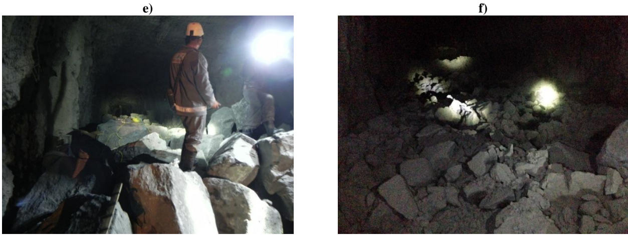
a, b, c, d, e – the appearance of oversized pieces before secondary crushing; f – the appearance of oversized pieces after secondary crushing
