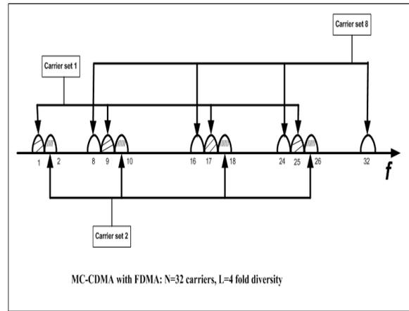
**Fig. 1. 32 carrier based FD-MC-CDMA**
