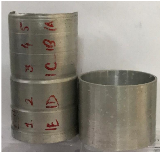
Fig. 4. Flow formed product and the preform
