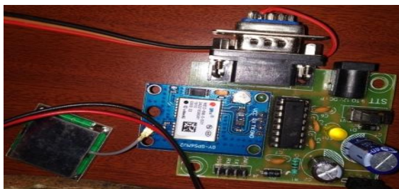
Fig. 8: GPS Module with EEPROM
