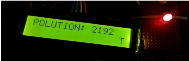
Fig. 17: Red LED turned on indicating fully unsafe state
