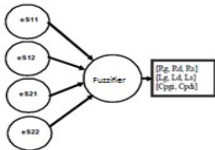
Fig 2. Fuzzy logic architecture for the proposed method for the extraction of extrinsic elements
