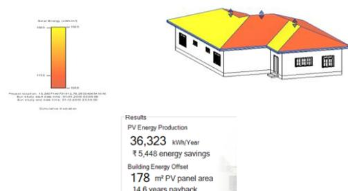
**Figure 17: Analysis of PV energy on sloping roof through software**
