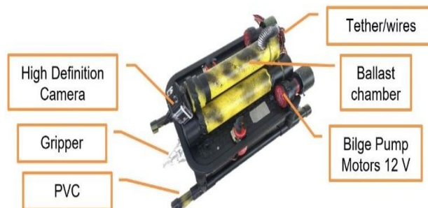
Fig. 2 Remotely Operated Unmanned Vehicle for Underwater Inspection (ROU-VUI)
