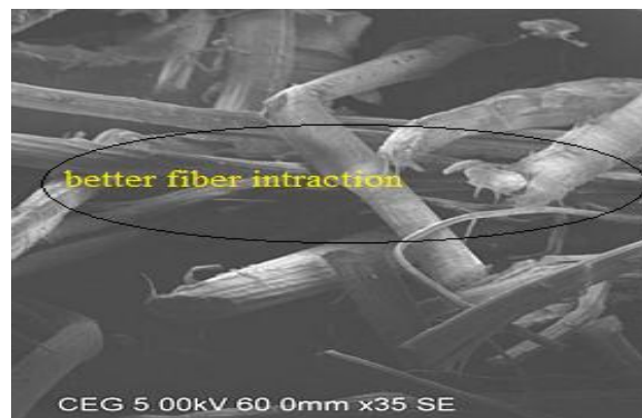
Fig-3 fractured specimen SEM image of treated fiber and matrix better interaction
