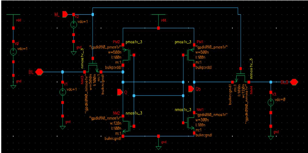
Fig.1. Single bit 6T SRAM Cell with write and read bit lines
