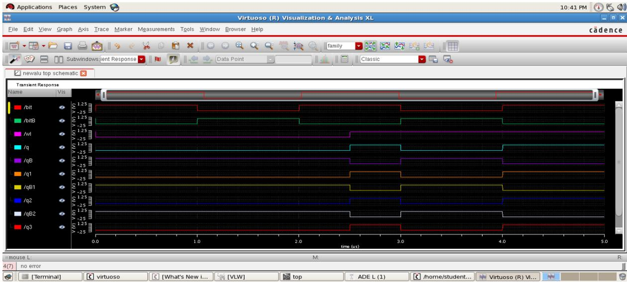
Fig 8: output waveform of 4bit 6T SRAM
