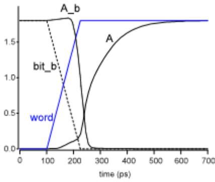
Fig.3. Write Margin Calculation from SNM.
