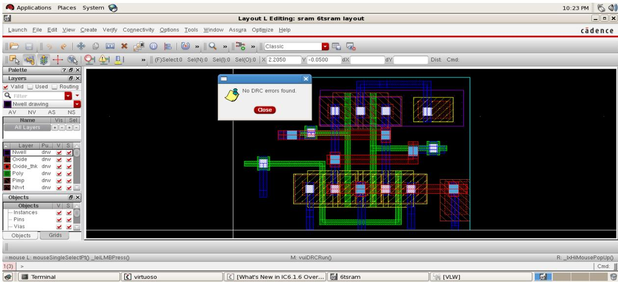
Fig 9(a): Layout desing of 6T SRAM with clean DRC
