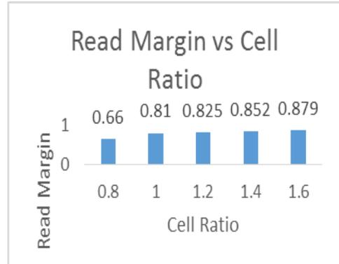
Fig.7. Graph of Read Margin vs Cell Ratio
