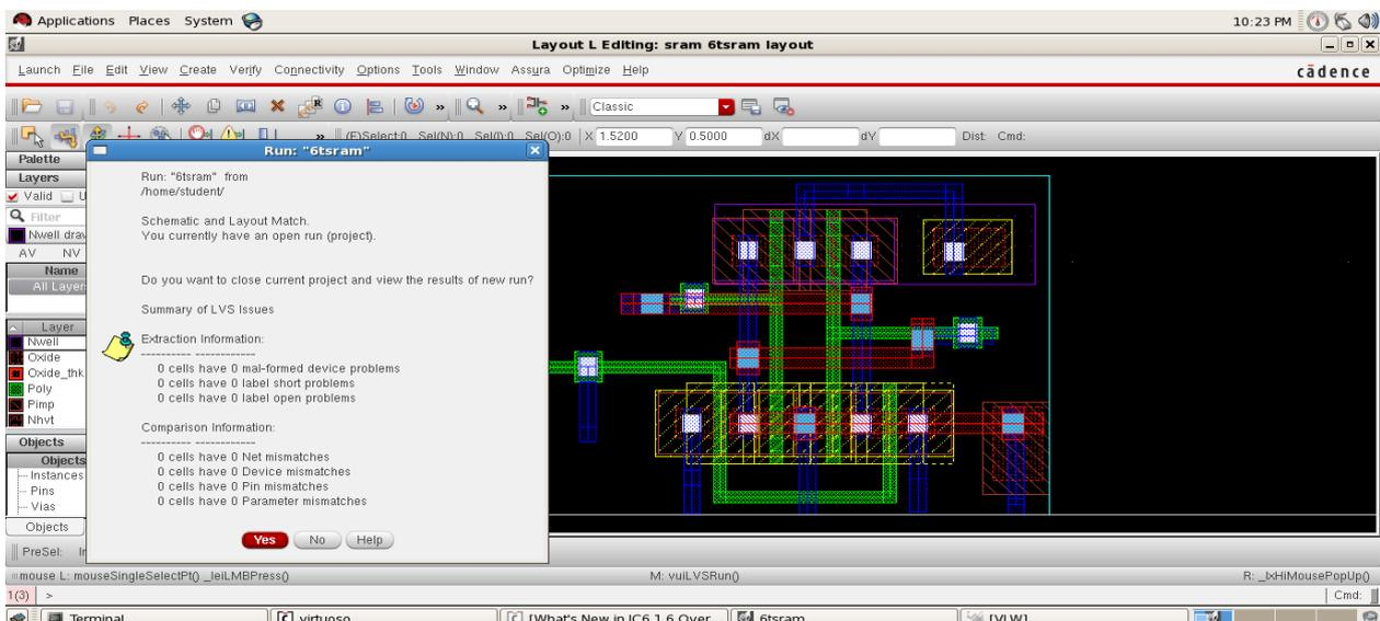
Fig 9(b) Layout design of 6T SRAM with clean LVS
