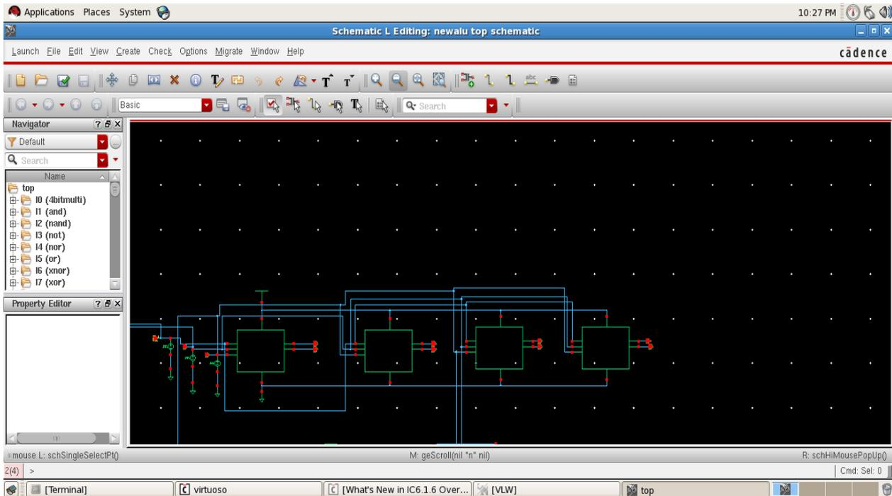
Fig 2: Top level design for 4bit 6T SRAM with write and read bit lines
