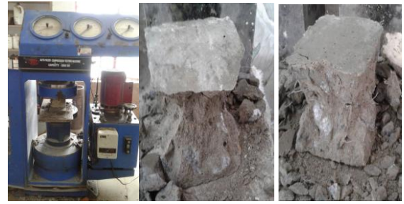
Fig. 4 Typical test set up and failure of specimens
