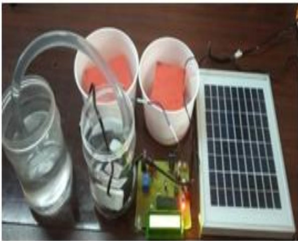
Fig. 9. Hardware setup of the proposed irrigation system using solar power under soil wet condition
