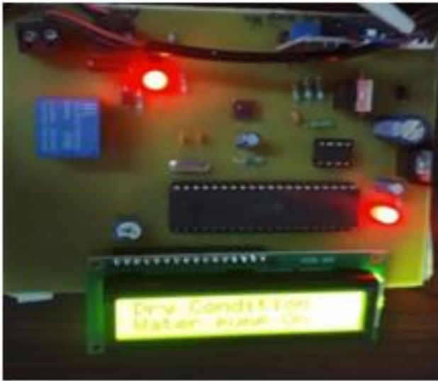
Fig. 8. Hardware setup showing soil dry condition and status of the pump in ON condition
