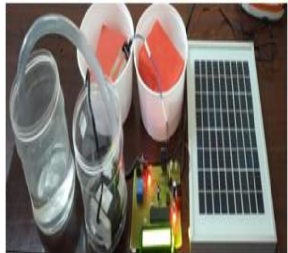
Fig. 7. Hardware setup of the proposed irrigation system using solar power under soil dry condition
