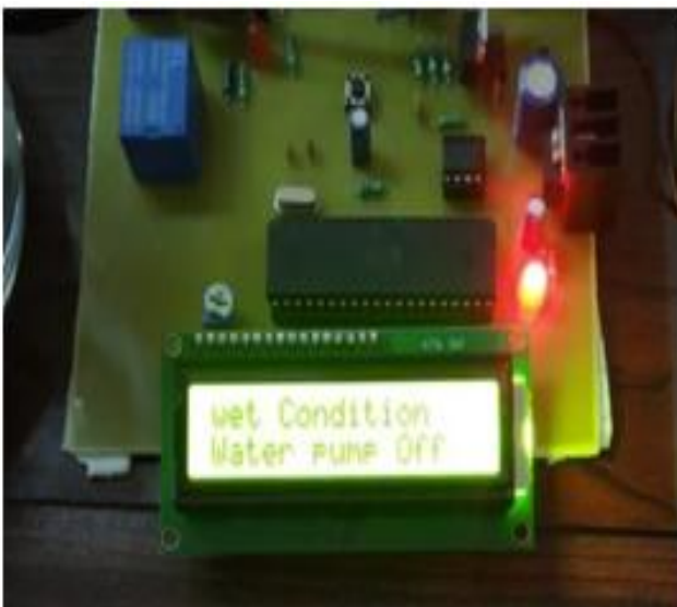
Fig. 10. Hardware setup showing soil wet condition and status of the pump in OFF condition
