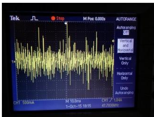
Fig-9 Chaotic output from electronic simulator observed at CRO with LE=0.2997 .
