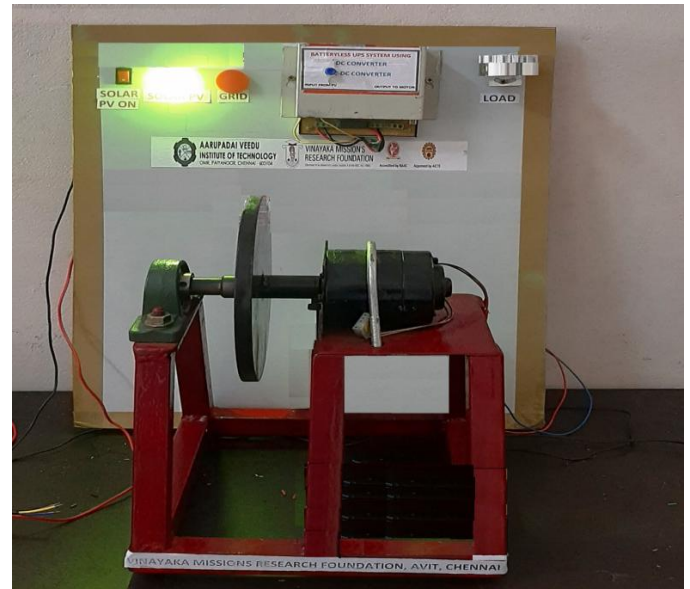
Fig. 7. View of the fabricated flywheel fitted with a motor
