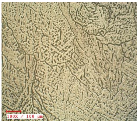
Fig. 7. Microstructure of Al-3.5% B4C MMCs.
