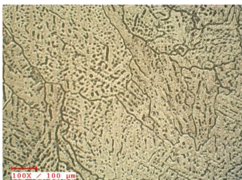
Fig. 9. Microstructure of Al-10.5 % B4C MMCs.
