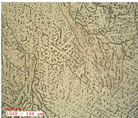
Fig. 8. Microstructure of Al-7.0% B4C MMCs.
