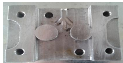
Fig. 15. Core and Cavity Plate
