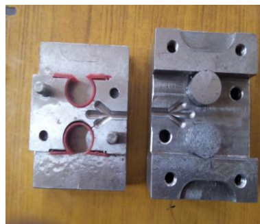
Fig. 17. After ejection of mould tool with component
