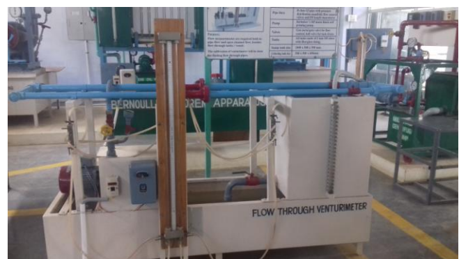
Fig. 2.Experimental setup of venturimeter
