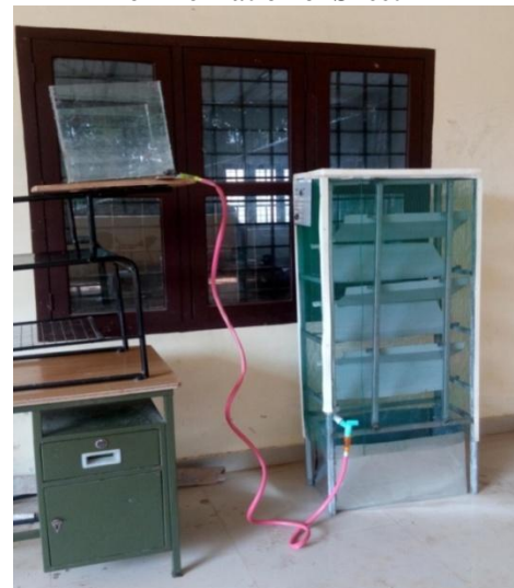
Fig 4: Provision for Changing Angle of Inclination of Sheet
