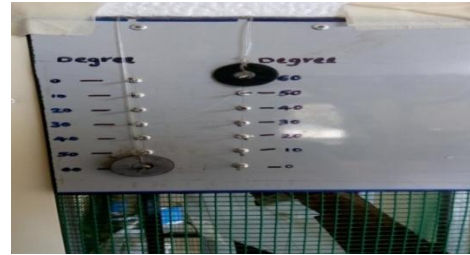
Fig 4: Provision for Changing Angle of Inclination of Sheet
