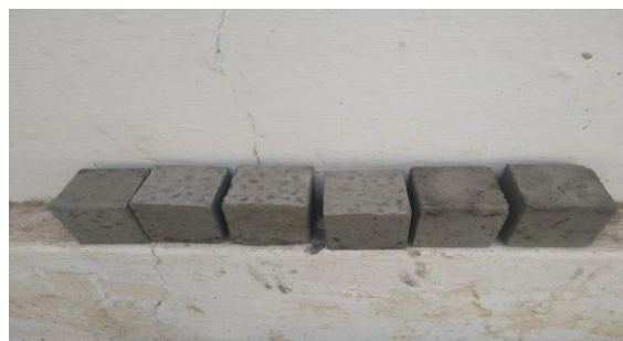
Fig.4. Cube specimens for acid resistance test
