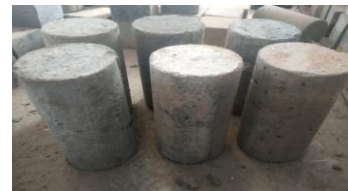
Fig.2. Specimens for water absorption test
