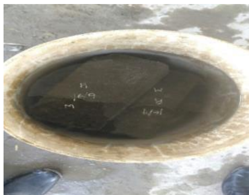
Fig 7.2 water absorption test on cement mortar bricks
