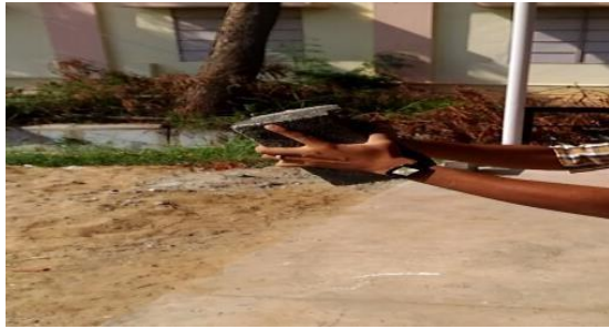
Fig7.3 Soundness test for cement mortar brick
