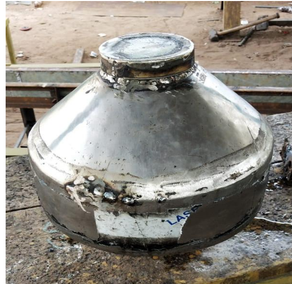
Fig. 4. Mixing chamber after welding
