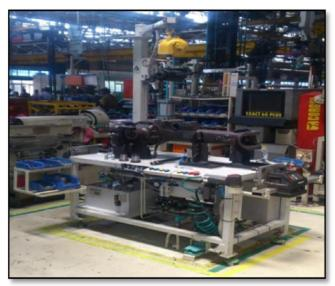
Fig. 17. New sub assy fixture Implemented in assy line
