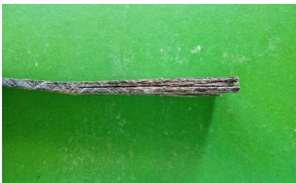
Figure 7. Photography image of delamination of 90-degree ply inter-lamina specimen with bio char.
