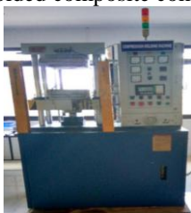
Fig 4. Compression molding machine
