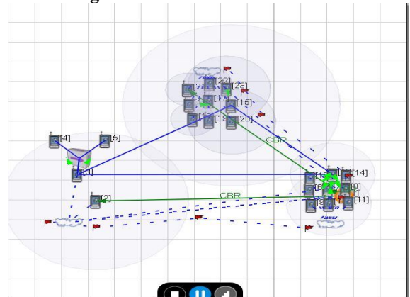
Fig. 3. Vertical handoff scenario between LTE and Wi-Fi heterogeneous network
