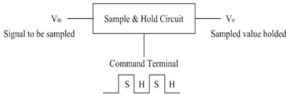
**Fig.2. Block diagram of Sample and Hold Circuit**
