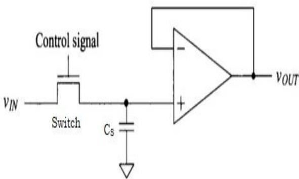
Fig.6. Schematic of S/H circuit
