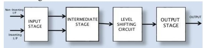
**Fig.4. Block Representation of Operational Amplifier**
