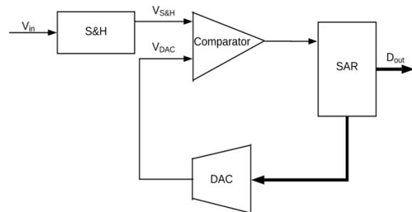
Fig.1. Block diagram of SAR ADC with sample and hold circuit
