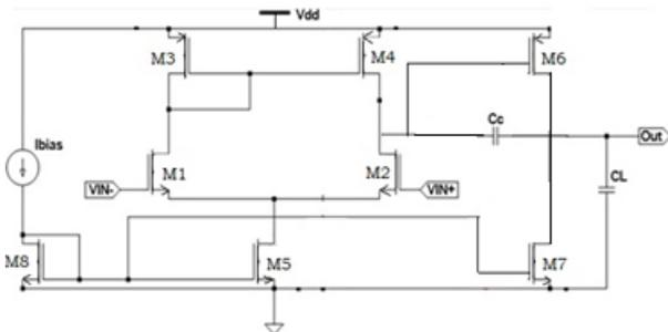
Fig.5. Schematic of Operational Amplifier for S/H Circuit
