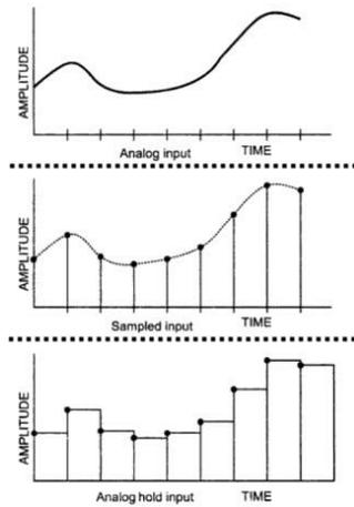
**Fig.3. Expected waveforms of sample and hold block**
