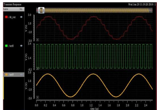
Fig. 9. Output waveforms of input, sampling and sampled Signal
