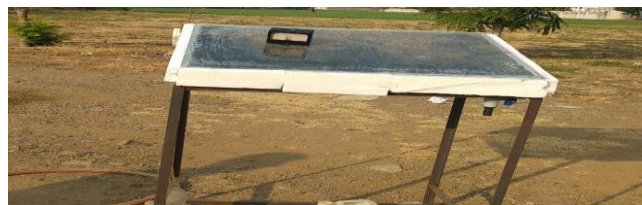
Figure 3.1 experimental solar still
