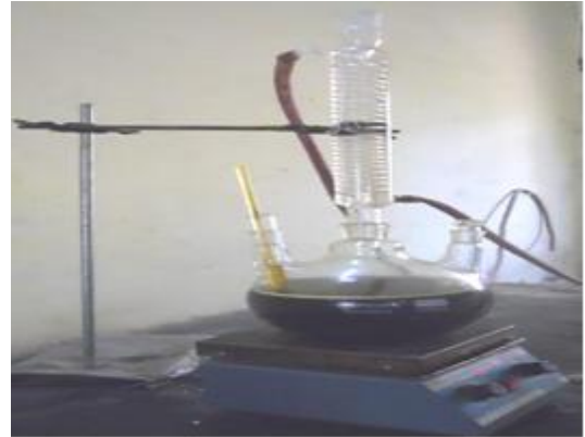
Fig.2.2 Experimental setup of transesterification process
