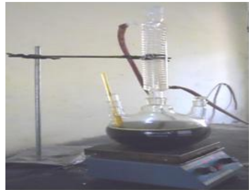
Fig.2.2 Experimental setup of transesterification process
