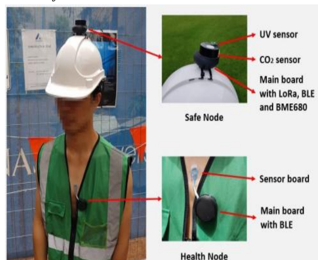
Figure 3. Health Node and Safe Node are attached to body and subject helmet
