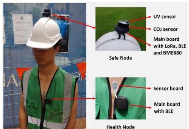
Figure 3. Health Node and Safe Node are attached to body and subject helmet
