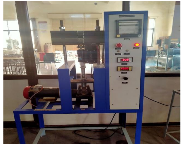
Fig.4: Shock Absorber Test Rig setup.
