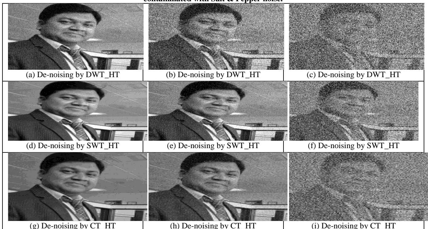
Fig. 3 De-noised images generated by different de-noising techniques using soft thresholding technique for DS dataset contaminated with Salt & Pepper noise.
