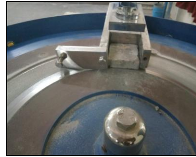
Figure 5: Abrasion test of tile
