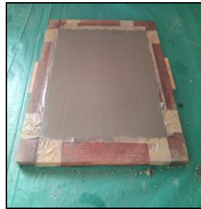
(a) Mesh-Reinforcement (b) Casted tile Figure 2: Casting of Tile
