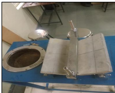
Figure 4: Flexural test of tile
