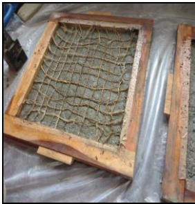
(a) Mesh-Reinforcement (b) Casted tile Figure 2: Casting of Tile
