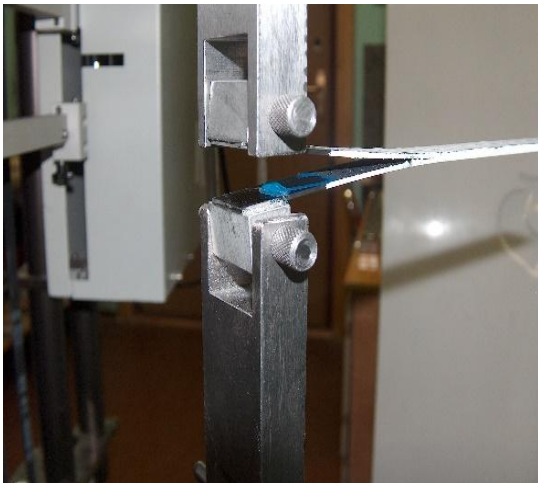
Figure 2 DCB Testing in progress
