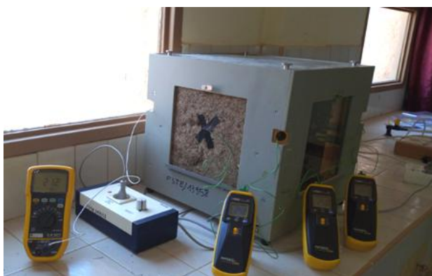
Fig. 2. Highly insulated thermal house method
