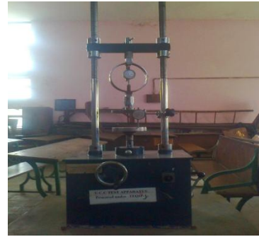
Fig.4. Unconfined Compressive Strength
