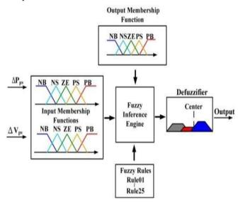
Fig:-5. Block diagram representation of Fuzzy Controller
