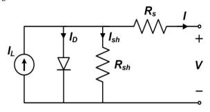
Fig 2: Equivalent circuit of solar cell
