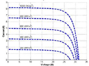
Fig:3. PV Characteristic of SPV Module
