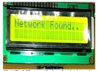
Fig.6. The LCD status after inserting the sim card
