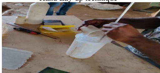
Mixing of Resin-Hardener-PU
