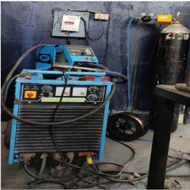
Fig 1: MIG Welding Equipment Used for Experiment
