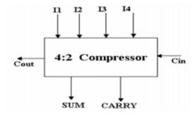
Figure 2. Block diagram of 4:2 compressor
