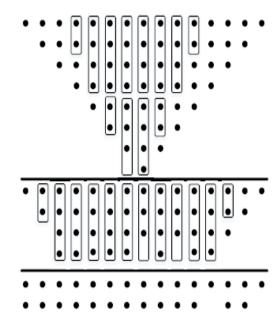
Figure 5: Dadda multiplier using proposed designs
