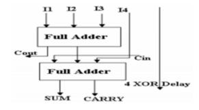
Figure 3. 4:2 Compressor design using Full Adder
