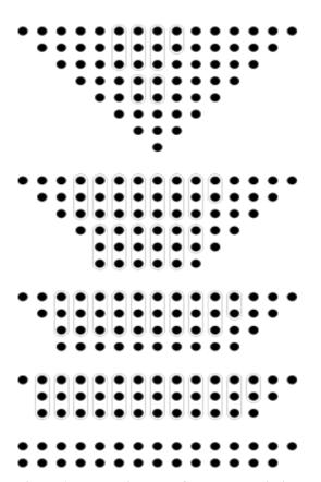
Figure 1: Block Diagram of Dadda Multiplier
