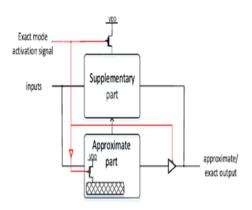
Figure 6: Block Diagram of proposed approximate 4:2 compressors. The approximate indicates the componenets, which are not shared between this and supplementary parts.
