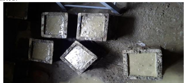
Fig(a) Casted cubes M_{40} grade of SCR
