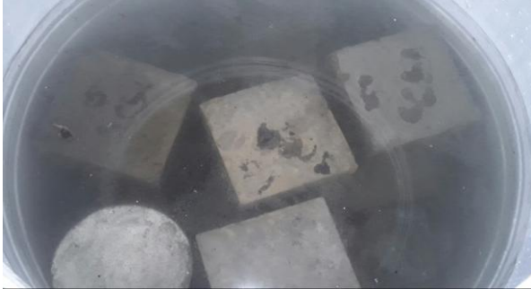
Fig (b) Curing Cubes of M 40 grade of SCR
