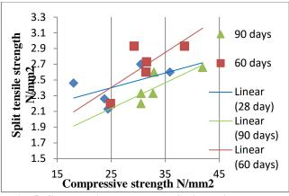
Fig. 5. Compressive strength Vs Split tensile strength
