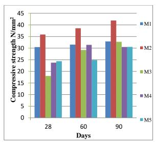
Fig. 3. Compressive strength for concrete cubes
