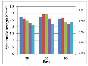
Fig. 4.Split tensile strength test
