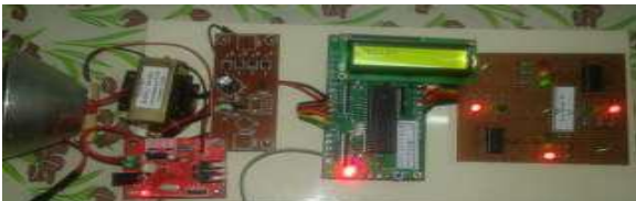
Figure 2 Transmitter for I2V mode Hardware setup
