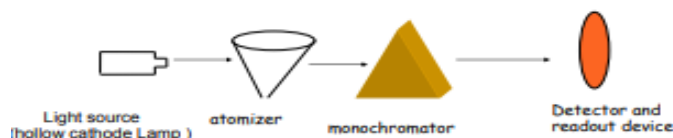
Figure 2 : Schematic Diagram of an atomic Absorption Spectrophotometer
