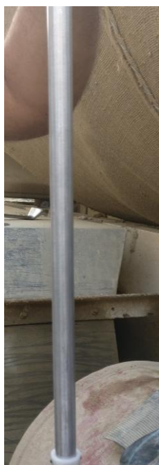
Fig. 7. Capacitive fuel sensor in the fuel tank.
