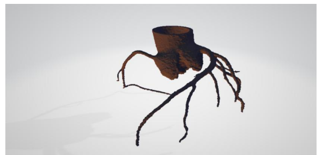
Figure1: The patient's image data is first converted into 3D Model and then the reverse engineering process extract a solid CAD model.
