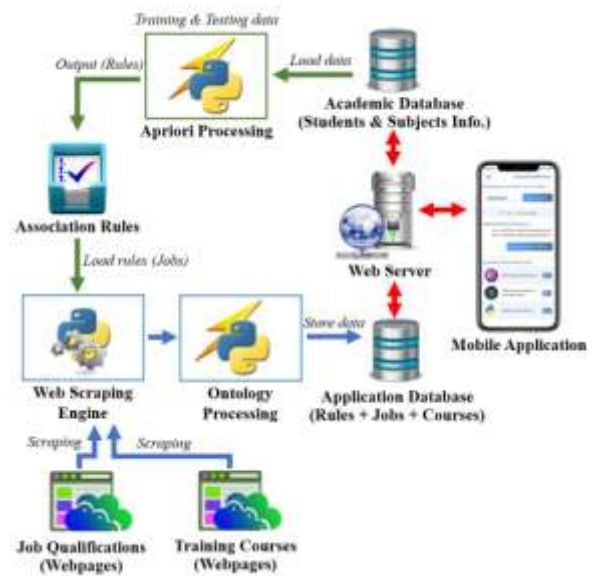
Fig. 2. The system architecture diagrams.
