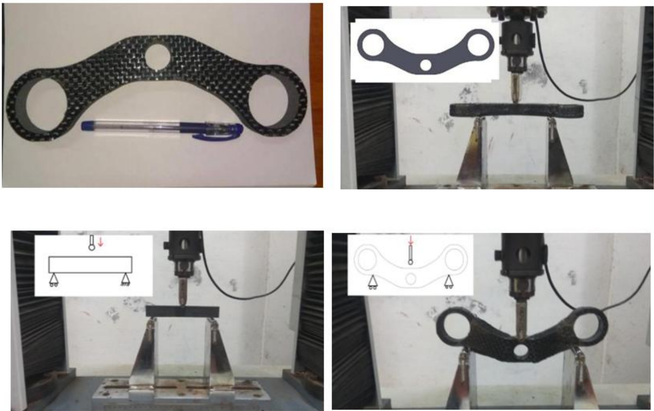
Fig. 6. Experimental set up for evaluation for data generation to validate FE model
