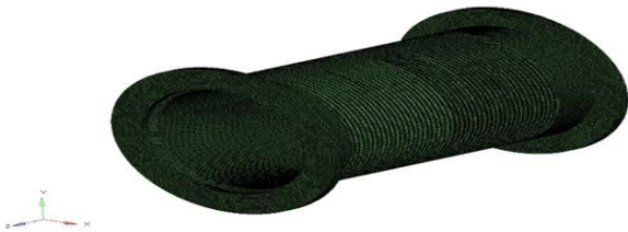
Fig. 3. Finite Element Model of Winch Shaft
