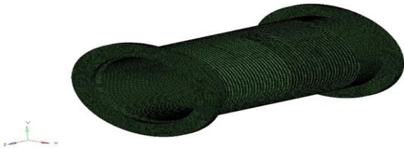
Fig. 3. Finite Element Model of Winch Shaft
