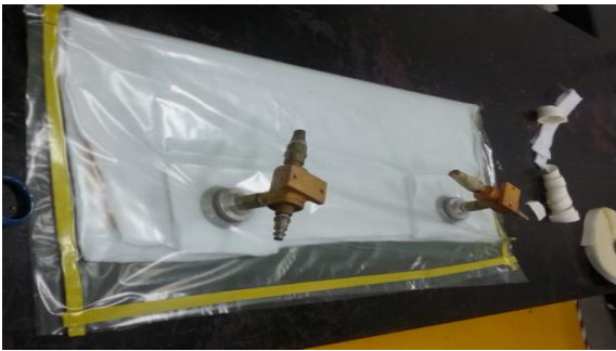
Fig. 6. Vacuum bagging process
