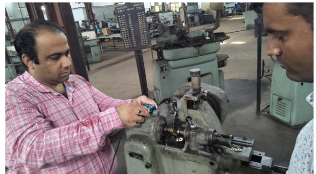
Fig 3: Industrial gear hobbing machine at Capstan Meters Pvt Ltd
